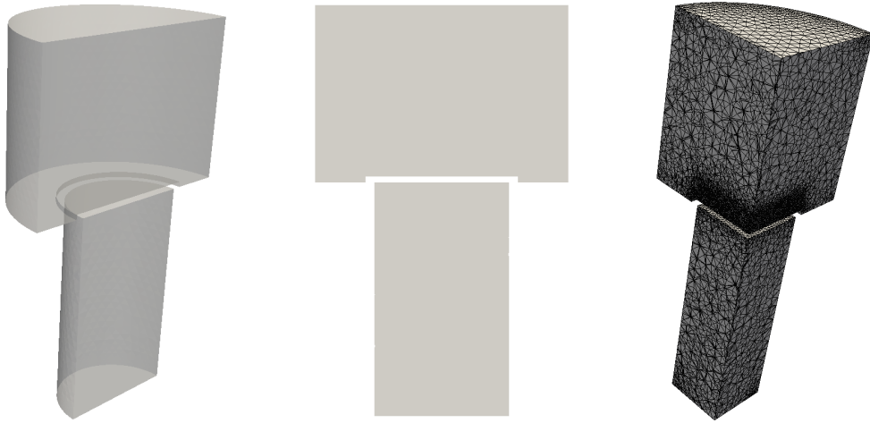
Figure 8.2: Numerical domain for L_1 = 0.12 m, L_2 = 0.088 m and l = 0.003 m. Left: Half of the numerical domain. Middle: 2D vertical slice of the numerical domain. Right: The mesh is superimposed on a fourth of the numerical domain.
