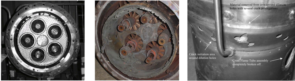
Figure 2: (left) Multiple swirled injector combustor. Reproduced from Goy et al. (2006). (middle) Damaged system. Perforates in the back plane chamber have melted. Reproduced from Goy et al. (2006). (right) Photograph of combustor damage caused by high frequency thermo-acoustic instabilities. Material was removed from the area around the dilution holes with several crack propagations. Reproduced from Sewell and Sobieski (2006).
