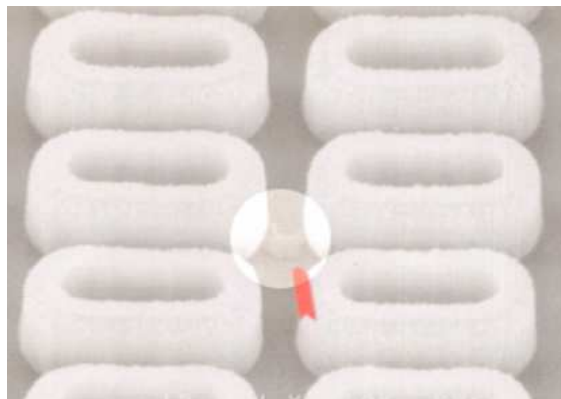
Figure 1.3: Residue induced intermittent fault in a DRAM chip [40]
