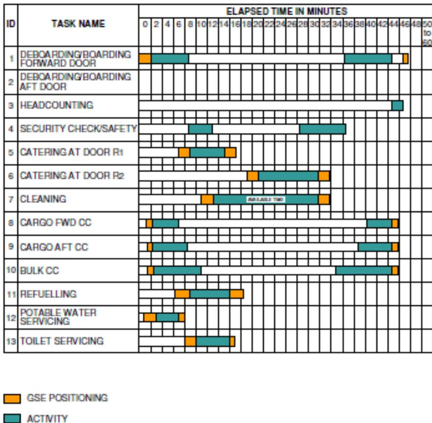
Figure I. 1: Full Servicing Turnaround Charts for an A320-100/ A320-200
