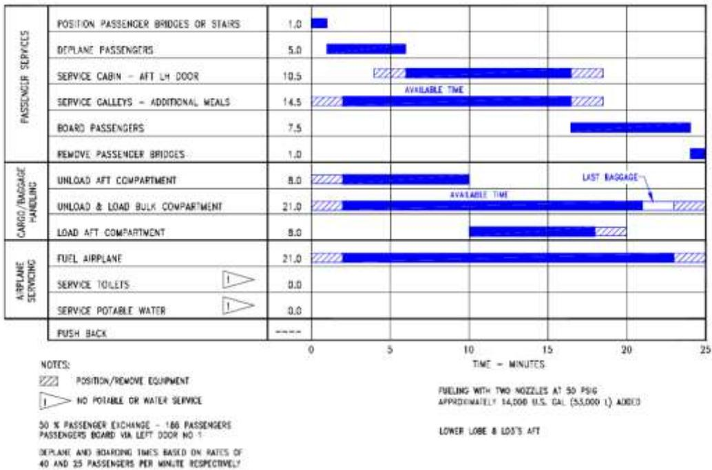
Figure I. 8: Minimum Servicing Turnaround Charts for a B777-200LR
