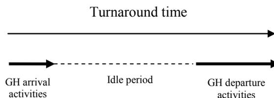
Figure 1.16: Turnaround with loose ground handling activities
