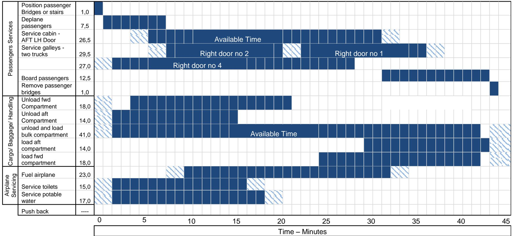
Figure 1.18: Typical durations of handling operations Boeing 777-200 [Boeing, 2009]
