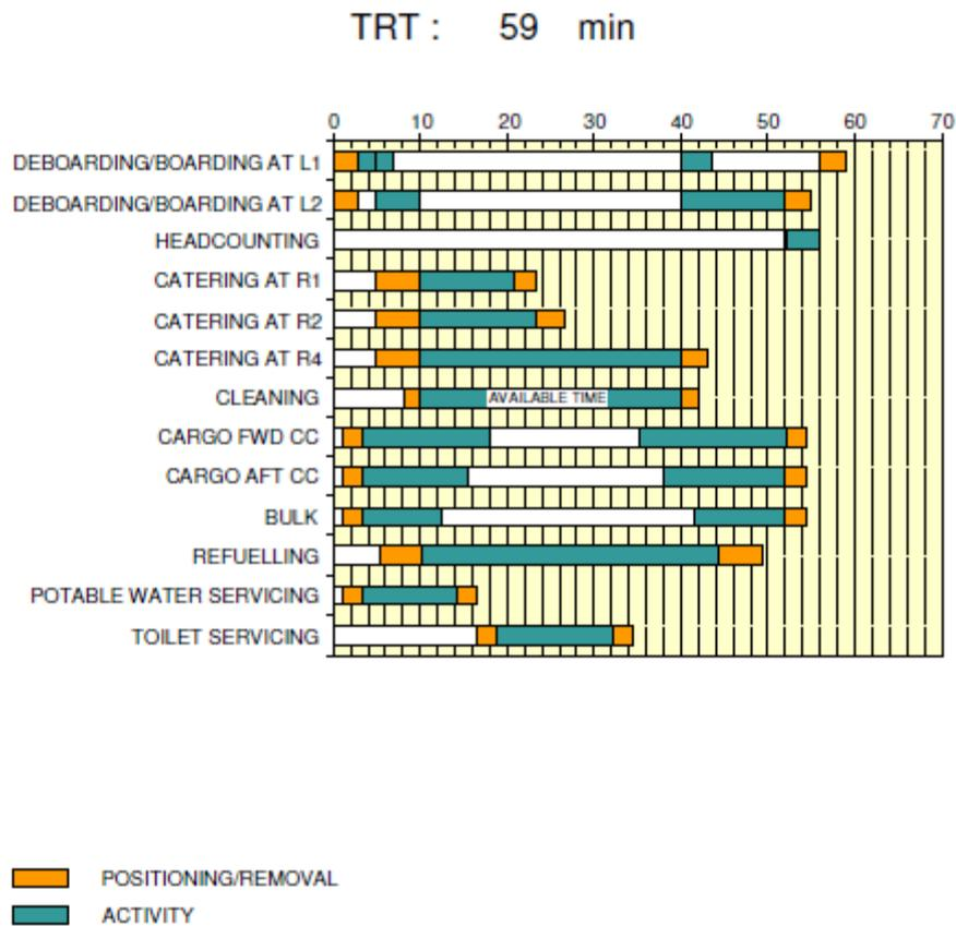
Figure I. 3: Full Servicing Turnaround Charts for an A340-200
