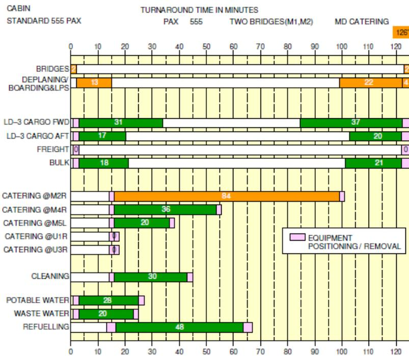
Figure I. 6: Full Servicing Turnaround Charts for an A380-800
