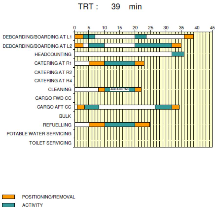
Figure I. 4: Minimum Servicing Turnaround Charts for an A340-200
