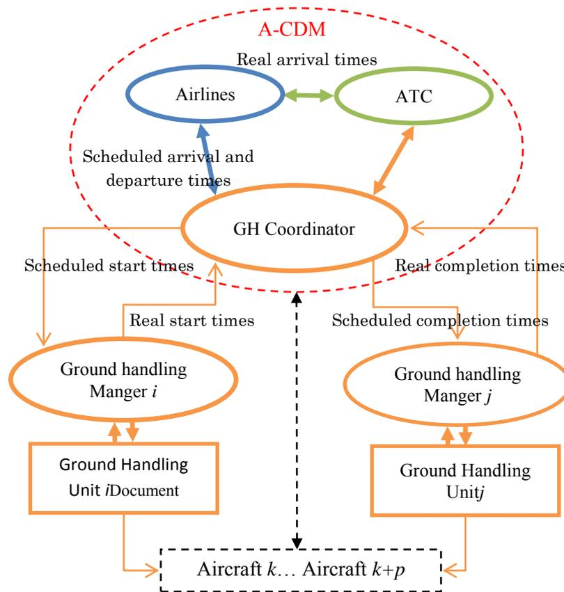
Figure 4.2 : Connection of A-CDM with Ground Handling
