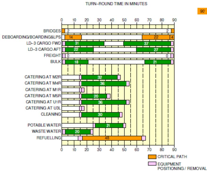
Figure I. 5: Minimum Servicing Turnaround Charts for an A380-800
