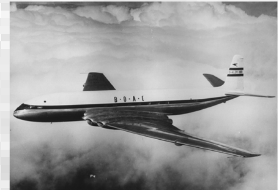
De Havilland Comet (1949): 1 st turbojet civil aircraft → much louder than propeller-aircrafts, WHY?
