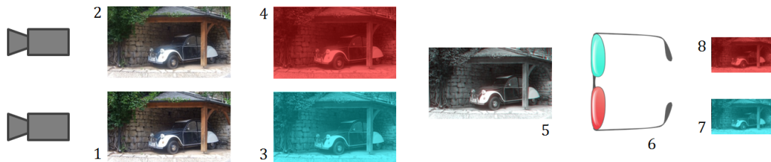
Figure 3.2: The functioning of a stereoscopic system using anaglyph glasses; adapted from [Sony 3D Television & Film 2010].
