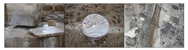
Figure 9.3 – Destructive damaging; a) cutting through one of the columns, b) and c) successive intersecting of prestressing tendons [VCE09].
