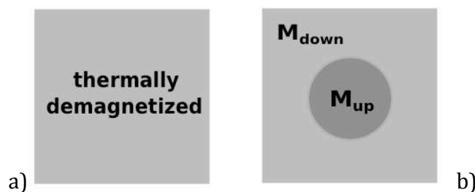
Fig. 5. 11 Schemes of the two types of magnetic surfaces that were imaged: continuous (i.e. non-patterned) film (a) and TMP film (b).
