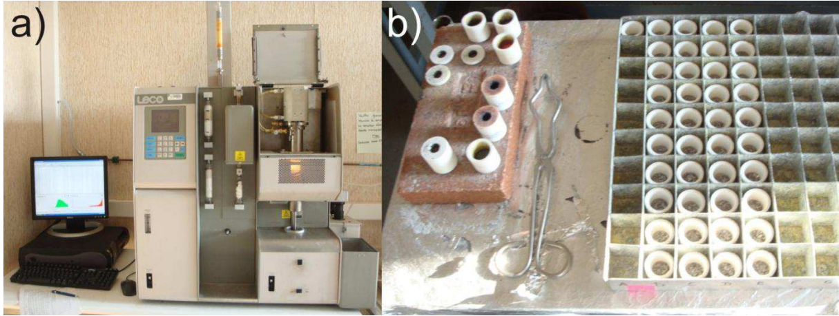
Fig. 3-5: Total and Organic Carbon analysis – a) Treated samples with HCl and b) LECO device
