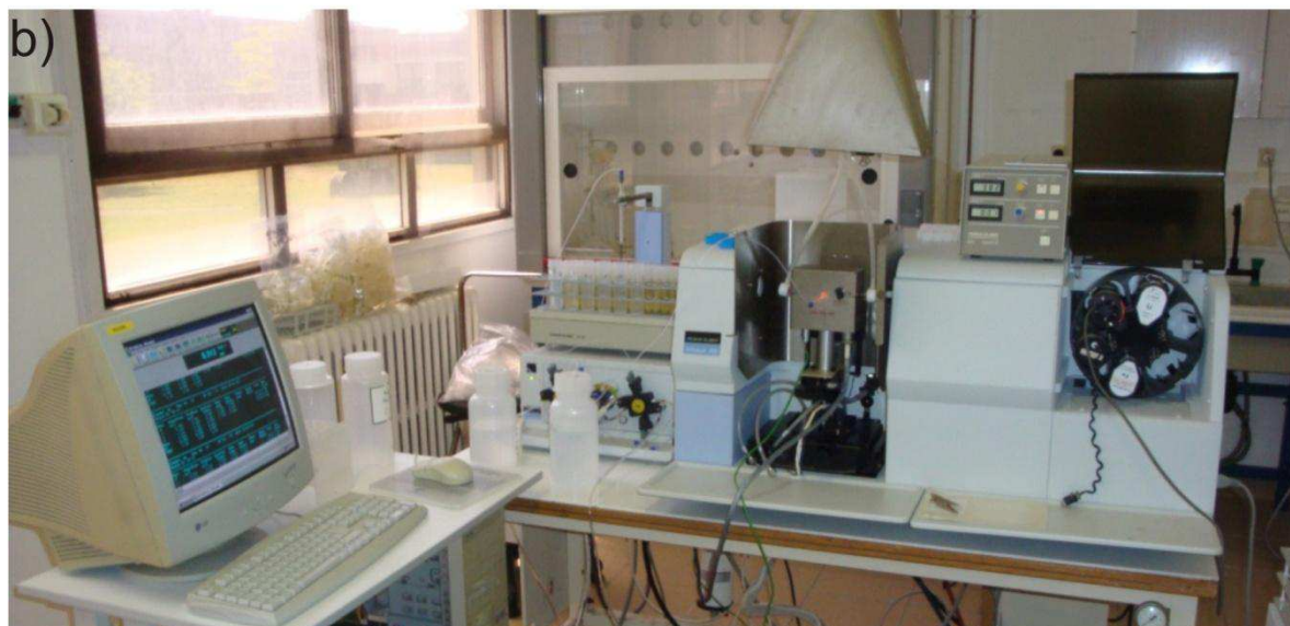
Fig. 3-8: Flow Injection Atomic Absorption Spectrophotometry, a) Schematic operation diagram of FIAS 300 (modified from Hineman, 2011) b) Measurement equipment at EPOC laboratory.
