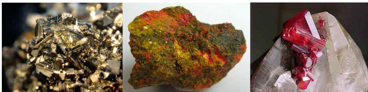
Fig. 2-5: Arsenic minerals. Left image, Arsenopyrite - \text{FeAsS} ( http://wisconsin geological survey.org ), middle image, Orpiment - \text{As}_2\text{S}_3 ( www.volcanol.fr ) and right image, Realgar – \text{AsS} ( http://webmineral.com ).
