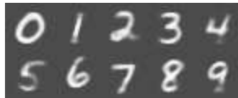
FIGURE 4.10: Imagery created from output unit decoding. Decoding from each of the 10 output units to the first layer produces a class-specific imagery with the appearance of a digit.
