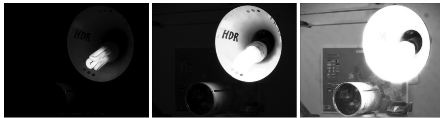
(a) Set. \Delta t_L = 0.094ms , \Delta t_M = 1,26ms et \Delta t_H = 5,36ms
