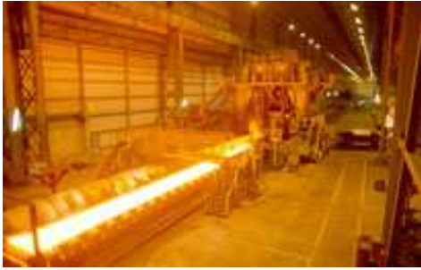
Reversing roughing mill and vertical edger
