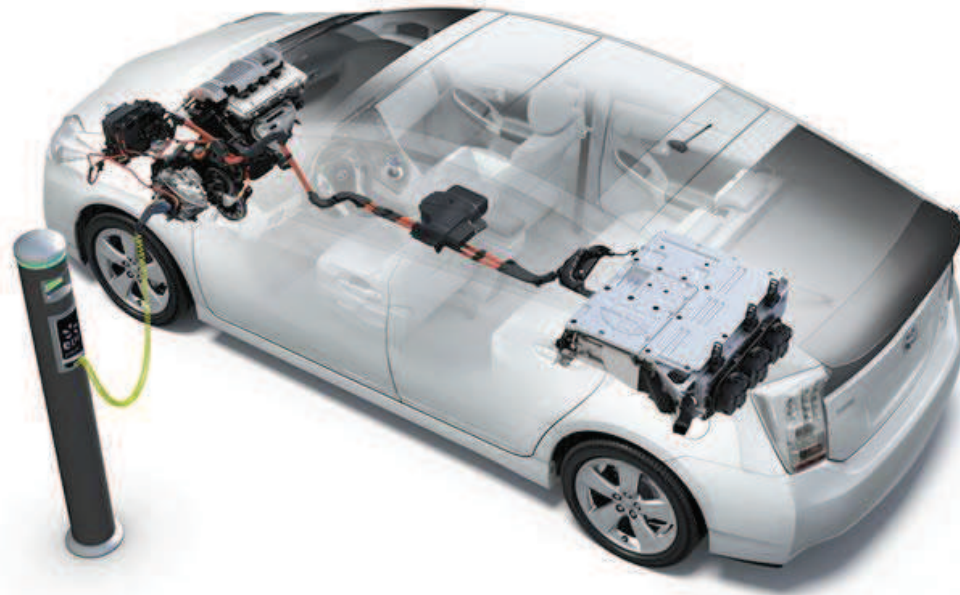
Figure 1.15 : Architecture Toyota Prius rechargeable.
