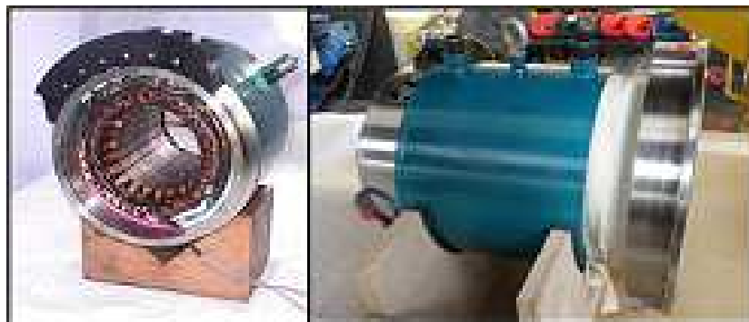
Figure 2.27: ECCE flywheel system homopolar synchronous machine [Mart05]
