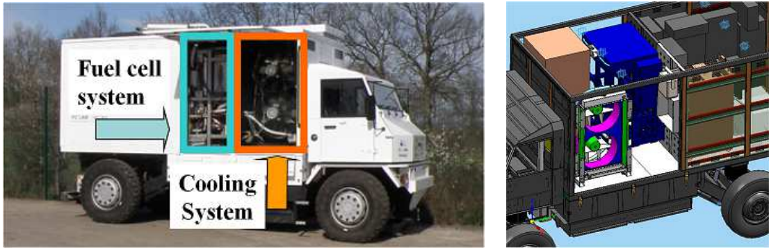
Figure 2.16: Fuel cell system implemented in ECCE
