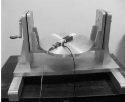
FIGURE 6.1: Photos of non-magnetic mechanical platforms. The figure on the left, depicts a motorized platform [80] and that on the right is a photograph of a non-motorized platform design [82].
