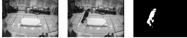
FIGURE 3.3 – Result of the moving object segmentation process. From left to right, background median model b_j , current frame i_j , segmented picture s_j for camera j .
