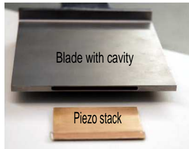
Figure 3.2: Blade with cavity and piezoelectric stack [119].
