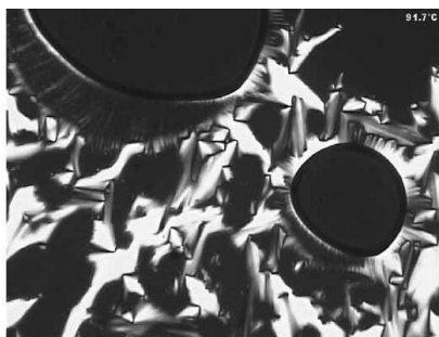
Fig. 2.8: Sm A* defect textures of dodecyl amide methylcarboxyl glucopyranoside at 91.1 °C ( \times 100 ) [147]
