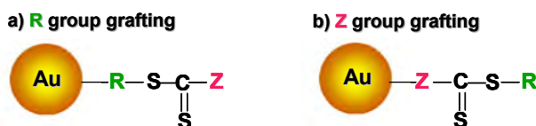
Figure III. 4: Grafting a CTA used for surface initiated RAFT via: a) R-group grafting; b) Z-group grafting.
