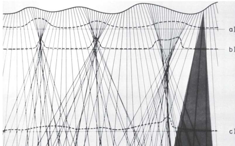
Figure 1.9: Graphic representation of the velocity bunching mechanism with respect to the wave steepness. The black solid line on top represents an ocean wave propagating in the azimuth direction. The rays leaving the wave surface are drawn with a slope relatively to the vertical which is proportional to the wave velocity component in the radar look direction, therefore having maximum slopes for rays starting near wave crests and minimum slopes for rays starting near wave troughs. The scatter points displacement induced by velocity bunching is proportional this slope. For the given wavelength, The impact of different wave heights on this displacement is represented by the greater distance between the transect and the wave profile. The black dashed lines plotted above each transect are the reconstructed wave profiles resulting from the velocity bunching effect. Transect (a) lies in the linear imaging region, while the images at transects (b) and (c) are strongly nonlinear. Taken from Hasselmann et al. (1985) .
