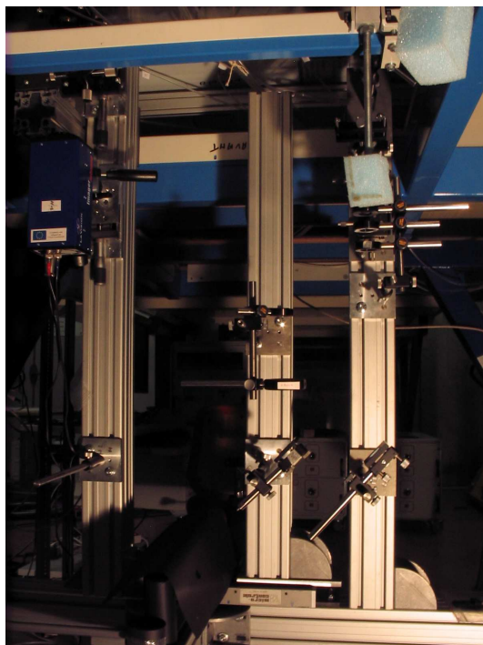
Figure IV.8: Photograph of the optical setup placed below the measurement station of the LML wind tunnel. Beam combiner and microscope objective cannot be seen properly because they are “hidden” behind a part of the tunnel structure.
