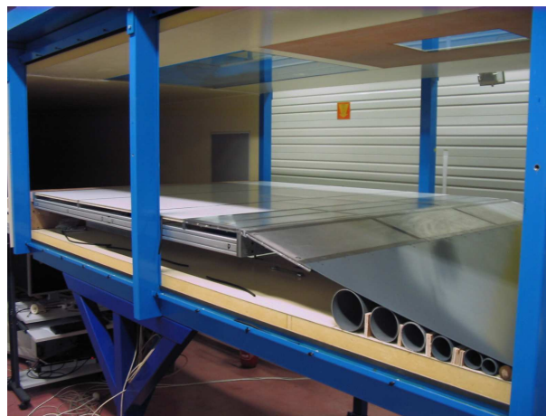
Figure IV.3: Photo of the measurement section. The bump model mounted for turbulent boundary layer control can be observed.
