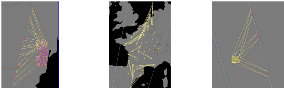
Figure 1.3: PLEIADES capabilities (from left to right) : adjacent regions, disjoint regions, tri-stereoscopic acquisition.
