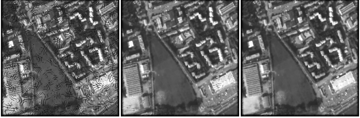
Figure 4.23: Experiment with spline degree zero (no deblurring) : gaps in the sampling set together with the conjugate gradient produce initial guess (left) with holes. If we force the Lagrange parameter the TV regularization fills these holes. Here we display an intermediate result (middle) where the holes are partially filled and a full convergence result (right) in which the holes have completely disappeared (remaining artifacts are due to the pixelation effect).
