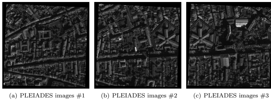
Figure 3.9: Test images (CNES copyrighted simulated PLEIADES images of Toulouse with resolution 0.7m). The couples have been rectified to epipolar geometry before the addition of horizontal microvibrations.
