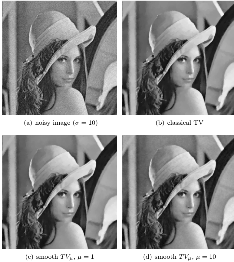
Figure 4.15: Experiments with the smooth TV proximal (denoising). For low smoothing parameters the difference is hardly visible ((b) vs (c)), but for higher smoothness the staircasing effect is clearly reduced ((b) vs (d)).
