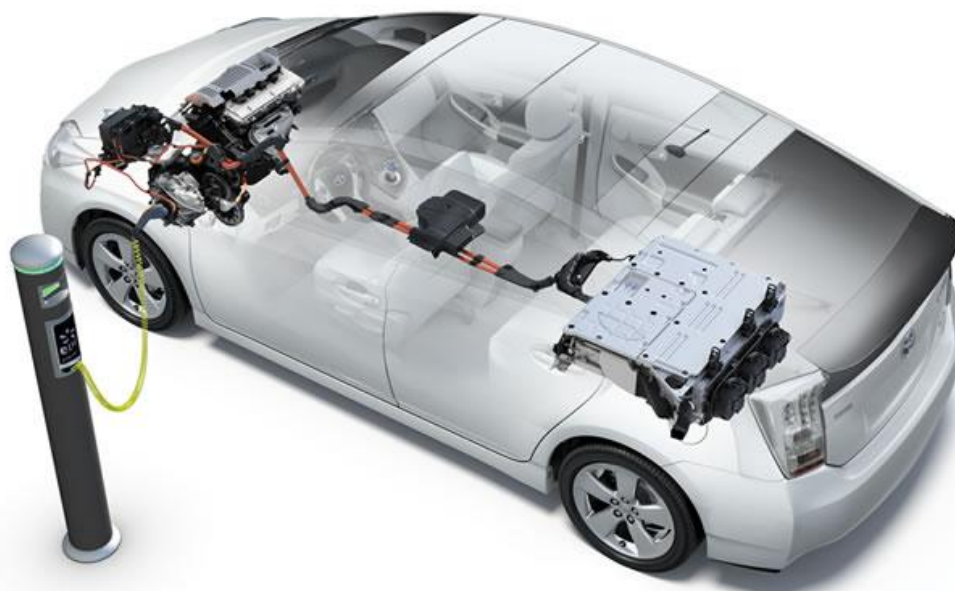
Figure 1.15 : Architecture Toyota Prius rechargeable.
