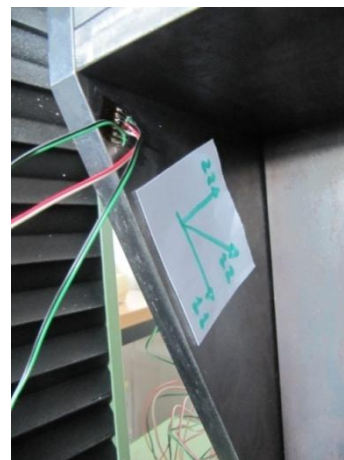
fig. II.64 - The strain gauge rosettes applied on the critical points of the apparatus. In the images are framed on the left the gauges 1 and on the right the gauges 2. Moreover the name of the axis is shown
