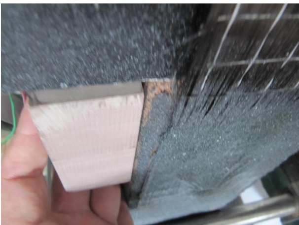
fig. II.81 - The template used to verify the 5[mm] distance between the fiber and the border of apparatus
