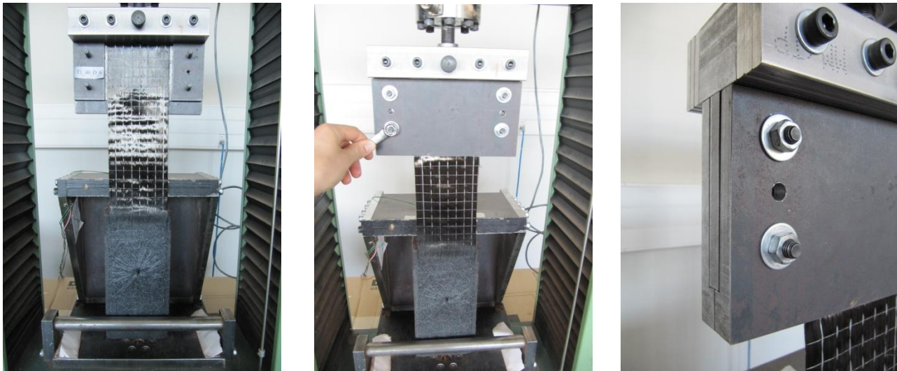
Figures II.80 - The steel grab reassembling and the @ plate clamping; three steps of the procedure
