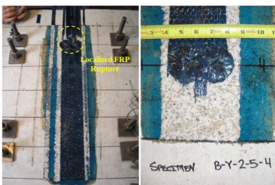
fig. I.50 - Failure of the specimen with two anchors placed across the width of the sheet [27]
