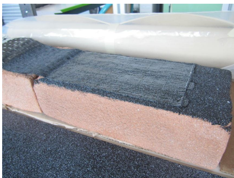
fig. III.20 - The speckle pattern onto the reinforced surface. The fire-brick specimen is drawn near the rubber sample characterized by homogeneous size spots.
