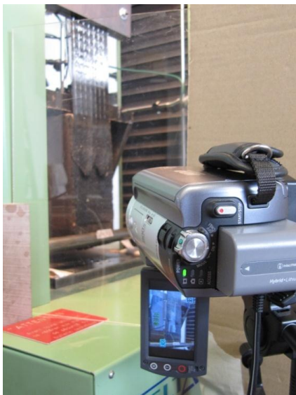
fig. II.85 - The Plexiglas foil interposed between the video camera and the specimen
