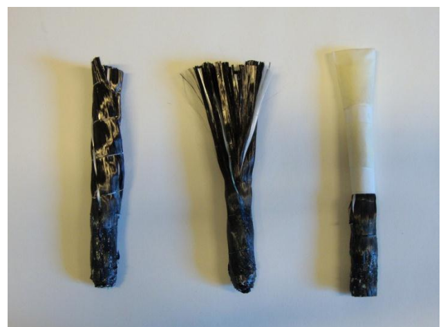
fig. II.21 - The impregnated anchor realized; on the right the anchor ready to be insert in the fire brick
