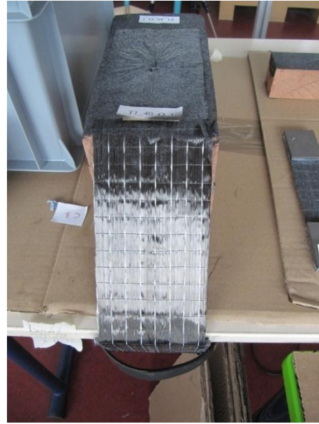
fig. II.74 - The device to stretch the fibers and block the plate without touch the adhesive
