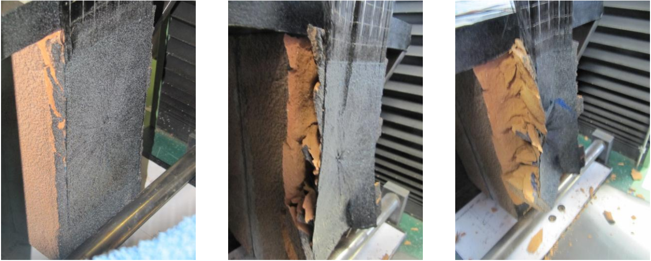
fig. IV.2 - The specimen during three test phases; in the left an image of the sample during the crack advancement (strokes BC), in the center a photo of the specimen after the total debonding fracture (strokes DE), finally, in the right a figure of the anchor detached from the CFRP sheet after the achievement of the P3.
