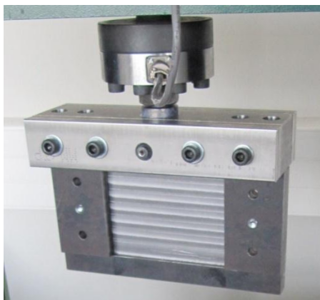
fig. II.78 - The configuration of the grab system disassembled
