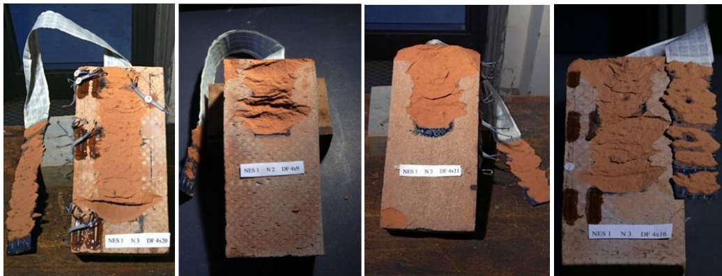
fig. I.29 - Failure mode, NES double shear tests (a courtesy of M. Fagone)
