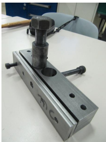
fig. II.68 - The horizontal piece realized to join the jaws to the pivot of the universal machine
