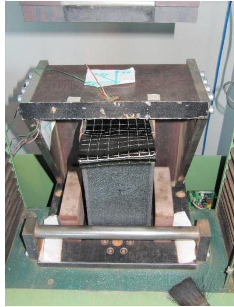
figures II.77 - The insertion of the specimen inside the steel apparatus (photo on the left ) and the reassembling of the Z steel lock using the two templates 70x140x40)
