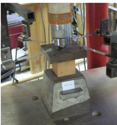
fig. II.5 Compressive test on a cube
