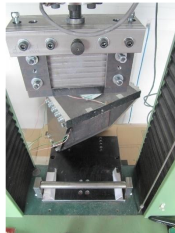
fig. II.76 - The alignment procedure of the Z box during the insertion of big size specimens
