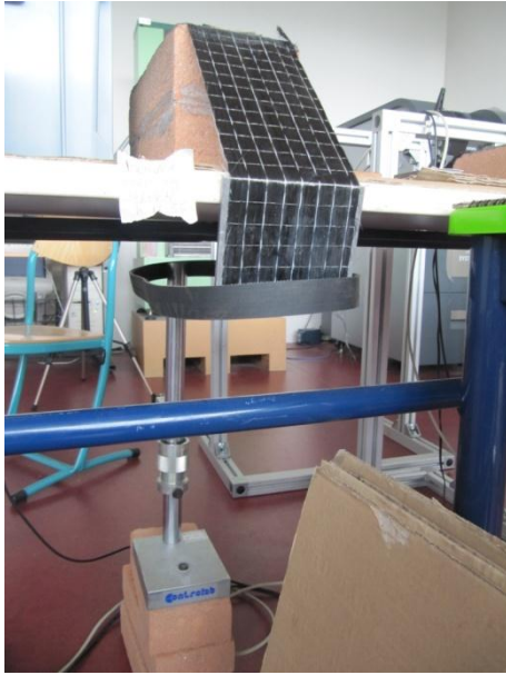
fig. II.74 - The device to stretch the fibers and block the plate without touch the adhesive
