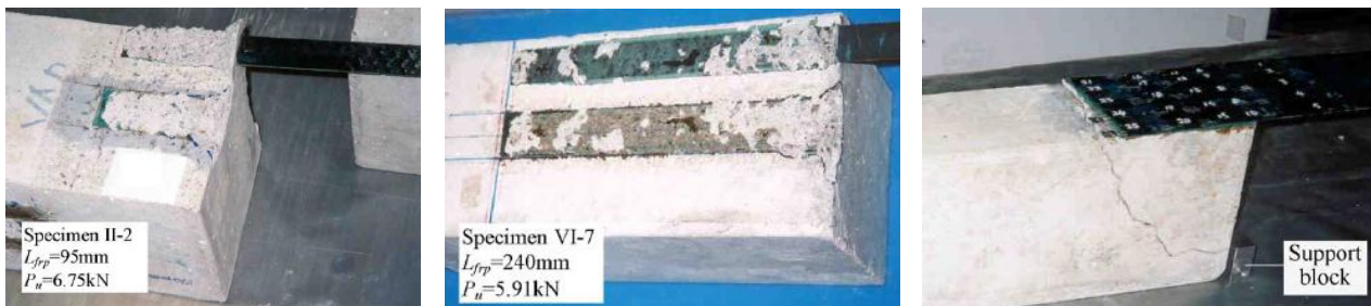
fig. I.25 - Failure modes in the Yao et al. experimental session [6]; a) Cohesive fracture, b) Adhesive fracture, c) concrete prism failure.
