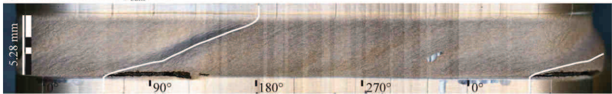
e) PP164 - 1170°C, \gamma_{\text{bulk}} = 3.9
