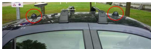
Figure 4.13. Antenna placement on the test vehicles.
