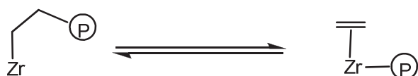
Scheme I.7: Ziegler-Natta polymerisation and depolymerisation mechanism over [\text{Zr-H}] , with \text{Zr-H} = [(\equiv\text{SiO})_{(4-x)}\text{ZrH}_x]/ x = 1 \text{ or } 2 . [9]
