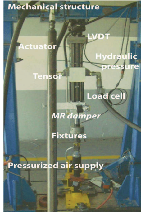
Figure 3.4: Experimental test-rig for MR damper parameter identification
