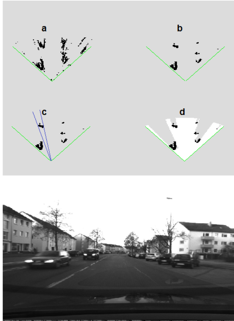
Figure 3.7: Steps to construct an occupancy grid for vision points. a) points projected on a grid, b) object points after noise removal, c) object cone for one object shown by blue lines, d) final occupancy grid for vision points. Image corresponding to these grids shown at the bottom.
