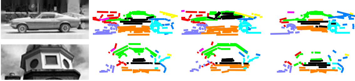
Figure 4.10: Positive and negative bags used by Multiple-Instance Learning (MIL) for the ‘car’ shape model: for each training image we compute a set of object instantiations, visualized as a part-level labelling of the image tokens. Through MIL we learn a classifier that accepts at least one instantiation per positive image and rejects all instantiations of a negative image.
