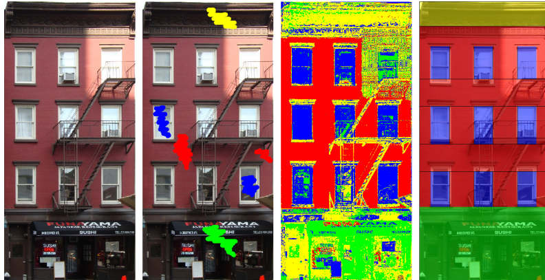
Figure 5.15: Grab-Cut -based facade parsing: we show, from left to right the original image, the user's brush strokes used to train a GMM classifier a pixel-wise segmentation using the learned GMMs, and the optimal parse delivered by our algorithm.
