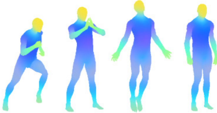
Figure 3.10: Invariance of the first three components of the HKS (shown as R, G, and B channels, respectively), for a shape undergoing isometric transformations.
