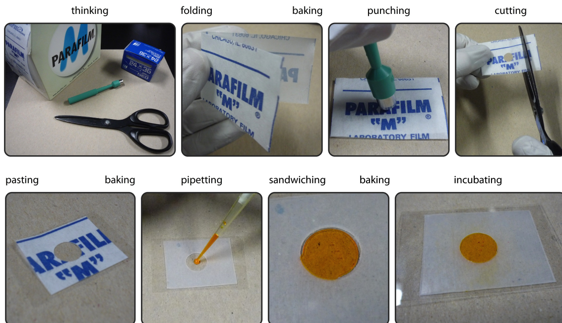
Figure 6.9: Making of Paraframe chambers.
