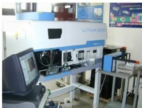
Figure II-15 : Appareil ICP – AES ULTIMA 2000
