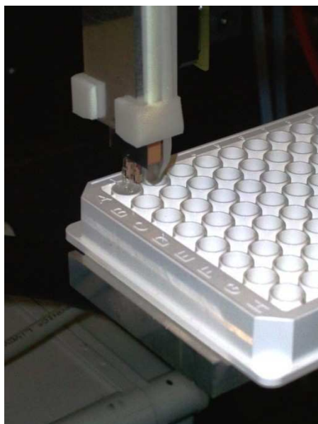
Figure 29: Crystal cryo-protection. The micro-gripper soaks the crystal in a cryo-protectant solution prior to flash-cooling.
