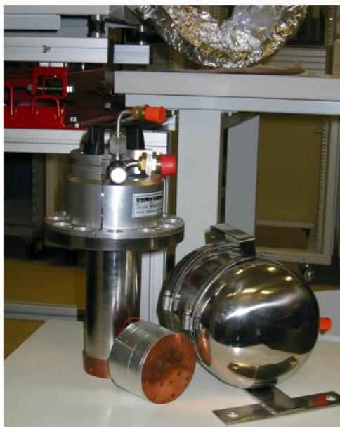
FIGURE 2.17 – Le PTR (Pulse Tube Refrigerator)
