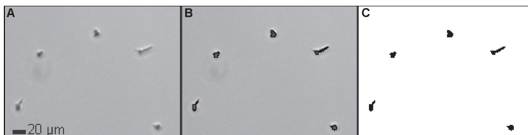
Figure 2.2: Cell contour detection. Detail ( \approx 10\% ) of one field of view obtained by bright field microscopy using a 4x objective lens (A) which is superimposed with cell contours identified by our ImageJ script (B). In (C) the corresponding binary image is displayed.
