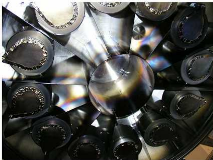
Figure III-2 – Photography of Plassys Sputtering machine.
