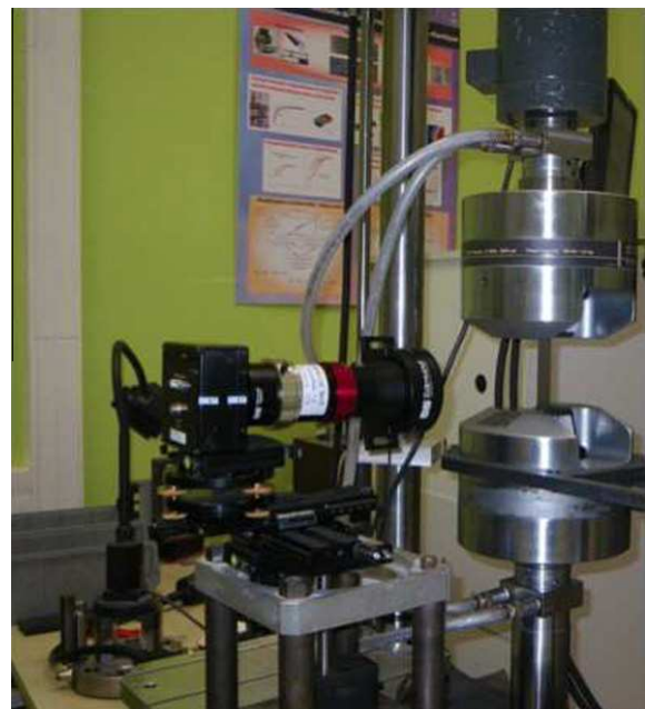
Fig. 2. Test configuration for the cyclic loading. A telecentric lens is used to minimize artifacts induced by out-of-plane motions.
