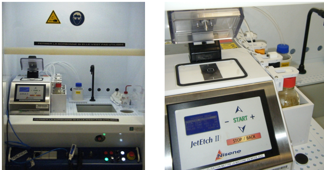
Figure 2.5: Chemical etching bench in MicroPackS laboratory and close-up on Nisene JetEtch II decapsulator.
