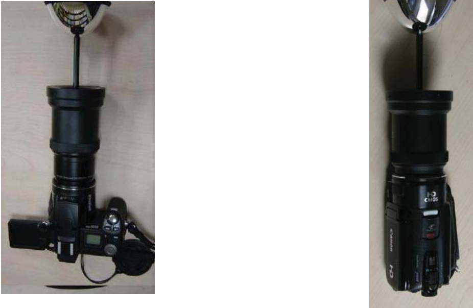
Figure 7.1: Catadioptric cameras used in experiments. Left: 0-360 mirror + Nikon Coolpix 8700; Right: 0-360 mirror + Canon Legria HFS10
