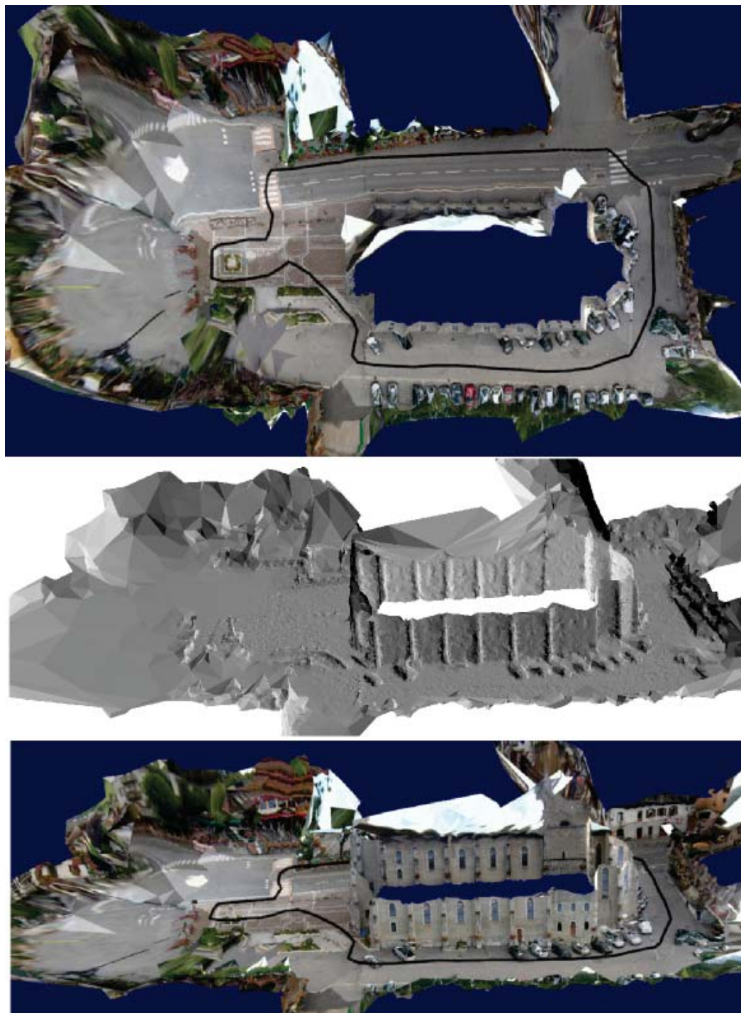
Figure 7.3: Overview of the batch surface reconstruction. Top and oblique views of the reconstructed surface (152k triangles), including triangle normals (gray) and trajectory (black).
