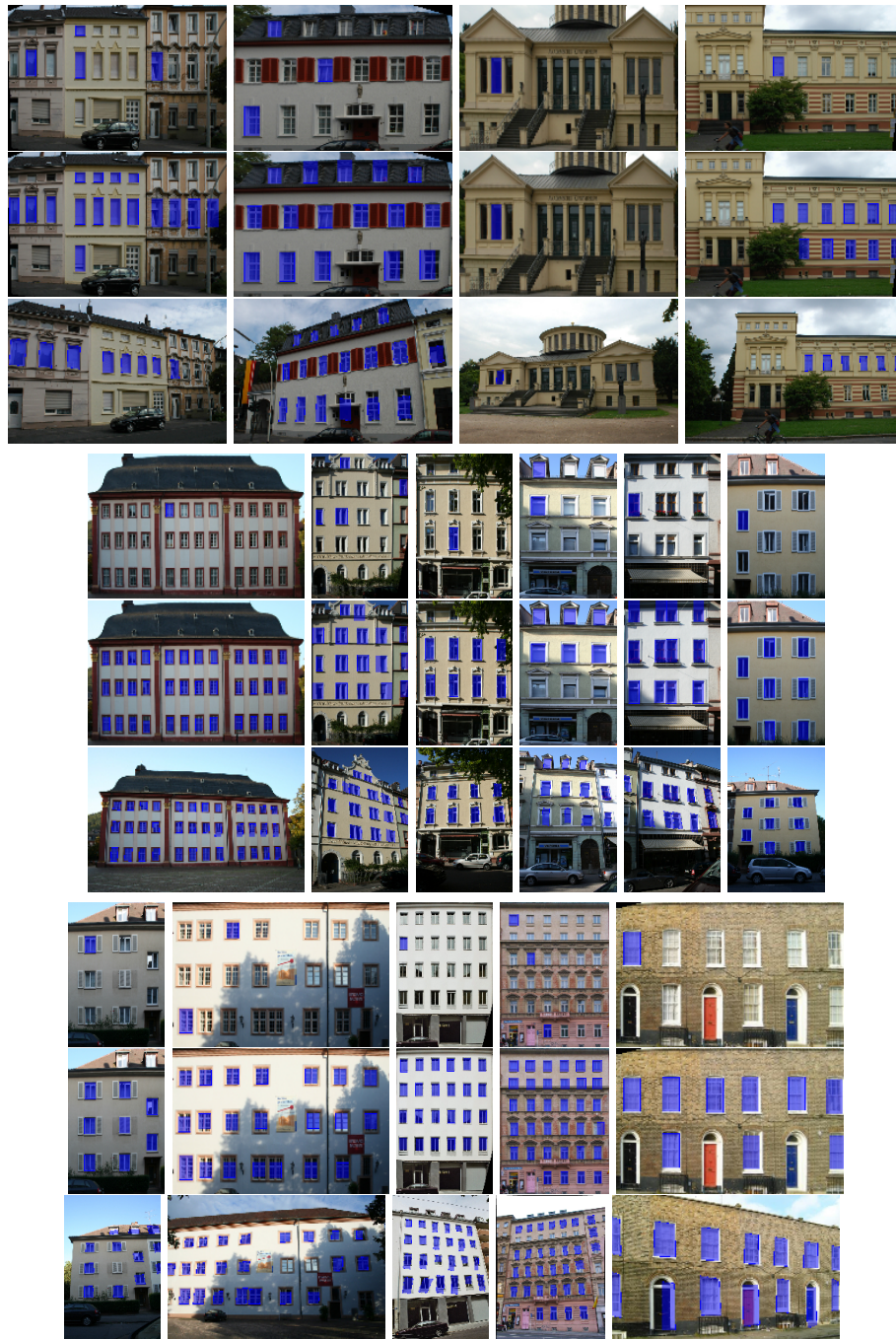
Figure 7.4: Window detection results on the eTRIMS dataset (2/2): input quadrilaterals, detections on rectified images, and detections on non-rectified images.
