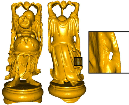
Figure 3.5: Stanford happy buddha : 380K vertices, 738K facets. Setting the tolerance parameter \sigma too high might create unwanted holes (inside the square).
