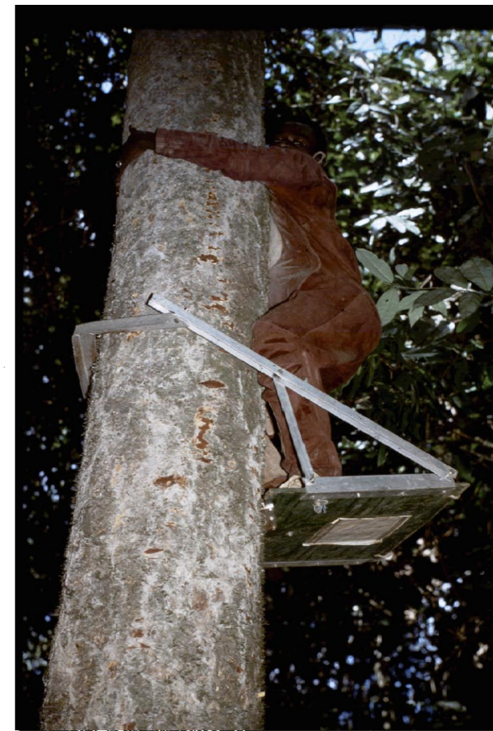
FIG. 1. The tree-climbing platform descending from 20 m height on a smooth tree trunk, in Gabon. Note the climbing marks of the gripping bar, along the trunk.
