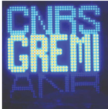
Figure 5.12: ICCD image with static mode of the array with mixed holes discharge reactors with 50, 150 and 100 \mu\text{m} diameters sub-hole arrays (bottom to top). (Image has false colours)
