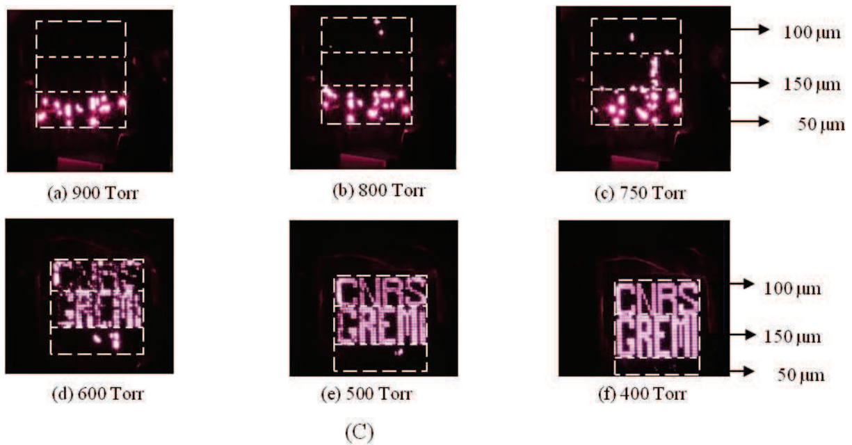
Figure 4.36: Effect of pressure variation in He gas environment on the arrays having different hole diameters 100, 150 and 50 \mu m on the same chip. (Dotted windows on the images indicate the border lines for different arrays)
