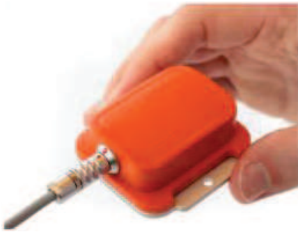
Figure 2.1. Centrale inertielle XSens MTi [XSens, www].
