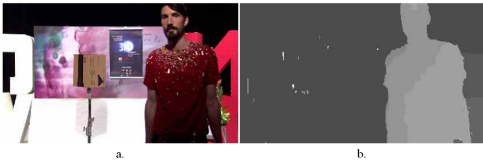
Figure 5.32. Disparity map extraction. (a) Original image; (b) Disparity map.
