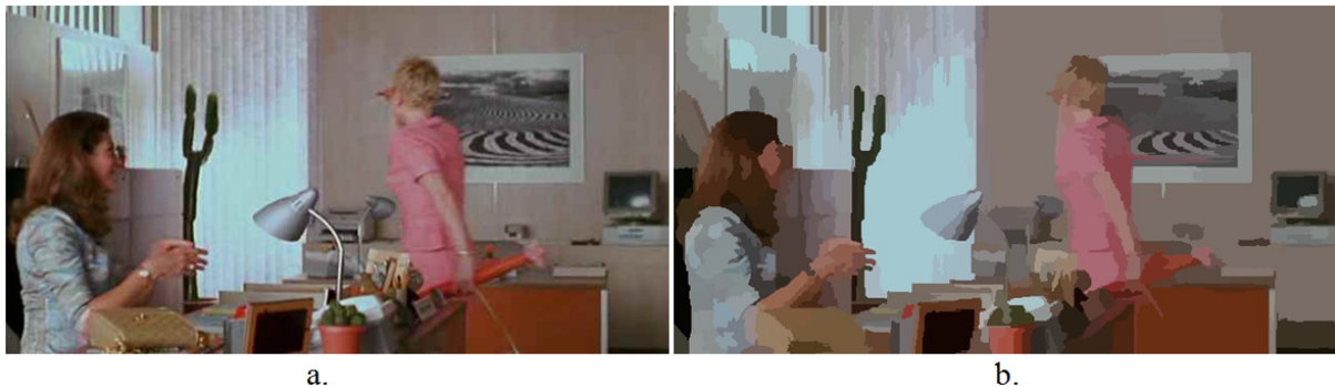
Figure 5.12. Image segmentation using the Mean Shift algorithm: (a) Original image; (b) Segmented image.
