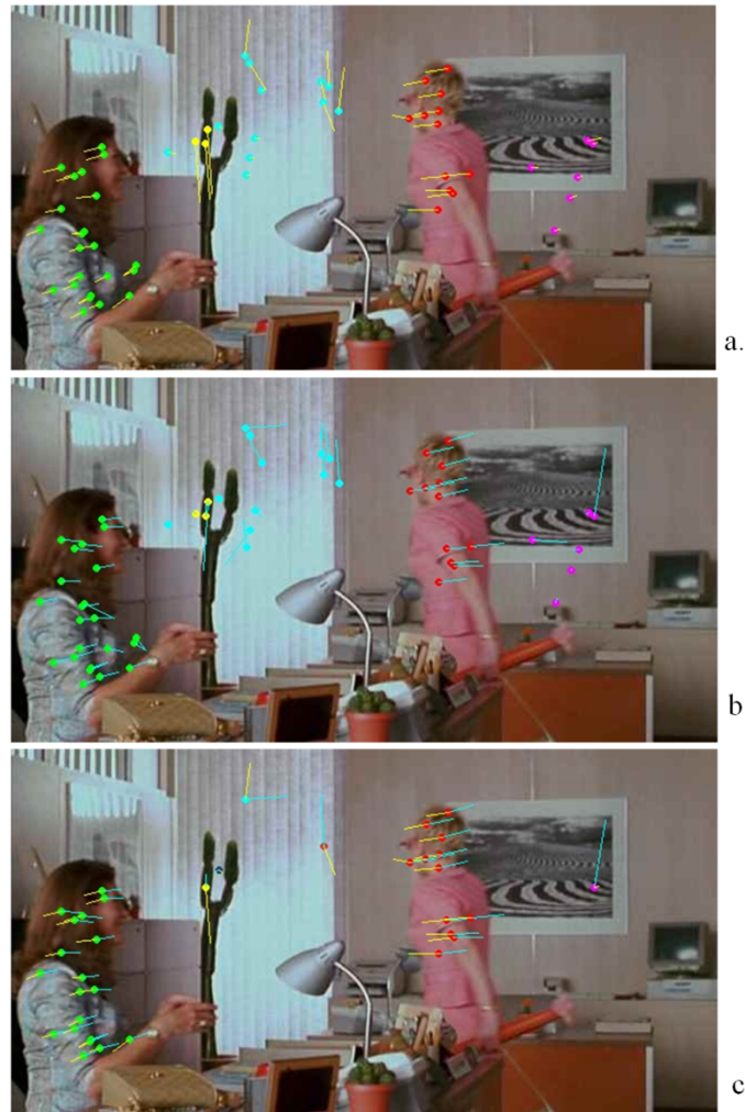
Figure 5.18. Motion vectors computed between.(a) Successive frames; (b) Predecessor frames; (c) Motion classes correction.
