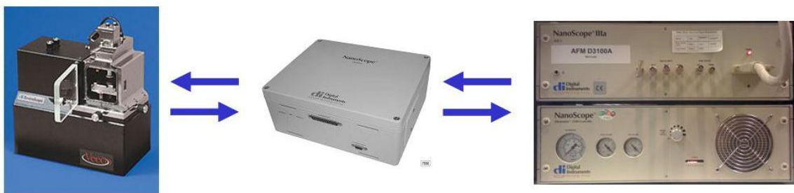
Fig. 3.2 The standard connection of EnviroScope™ only enables amplitude modulated Tapping™ mode AFM and Lift-mode KFM. From left to right: EnviroScope™ AFM, Quadrex and NanoScope IIIa electronics.
