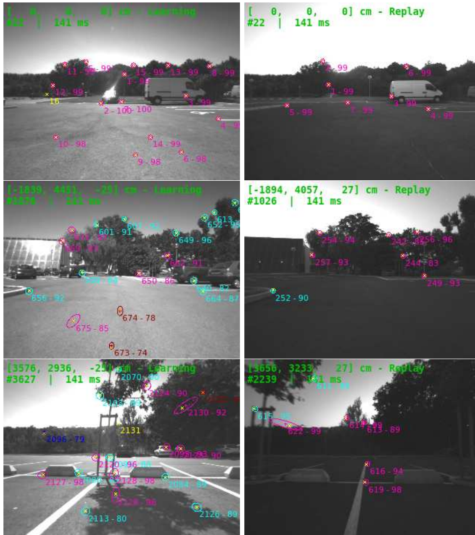
Figure 5.7: Learning and Replay experiment: images acquired on the same area. (left) learning-mapping step; magenta : IDP landmarks; dark red : IDP landmarks not observed in the frame; cyan : euclidean landmarks; dark blue : euclidean landmarks not observed in the frame. (right) replay-localization step; magenta : initial projections of 3D points from the learned 3D map; cyan : projected and matched points using for localization.
