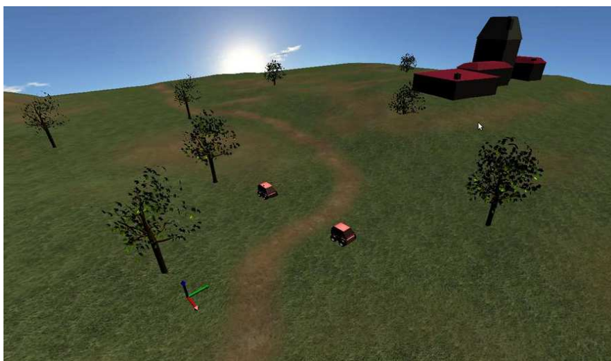
Figure 5.1: The MORSE Simulator: a domain independent simulator, where virtual robots can interact with a 3D environment, using sensors and actuators that behave in the same way as their counterparts in the real world.
