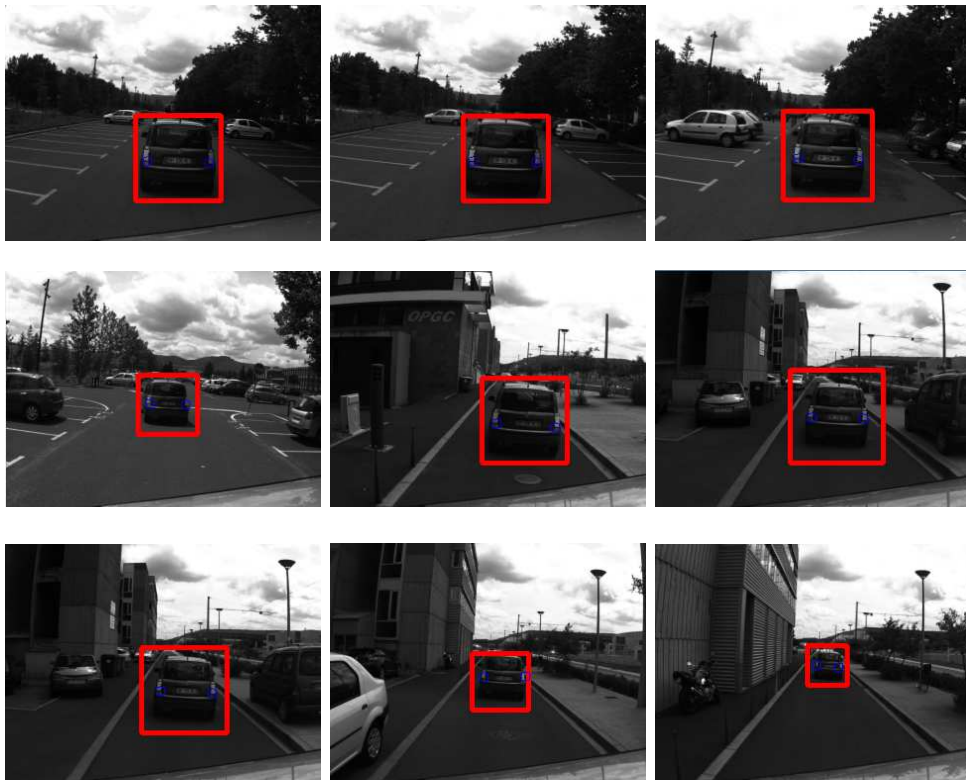
Figure A.13: Representative snapshots of the sequence. In the image view, red square is the leader vehicle detection; blue circles are pairs of features-light detection. The leader vehicle has been successfully detected and tracked. The pose estimation is based in the pairs of light detection.
