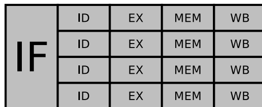
FIGURE 1.5 – Instructions executions on a 4-instructions VLIW processor
