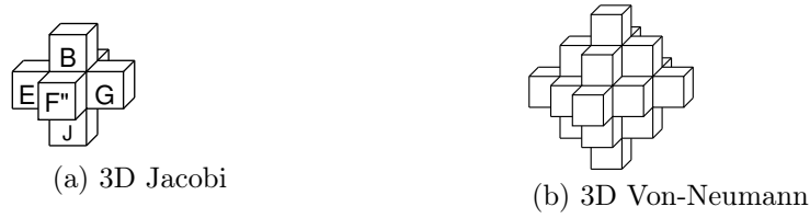
FIGURE 3.12 – Shapes of the studied stencil. (a) Shape of a 3D jacobi stencil. (b) Shape of the convex envelope of a 3D Von-Neumann neighbourhood of range 2.
