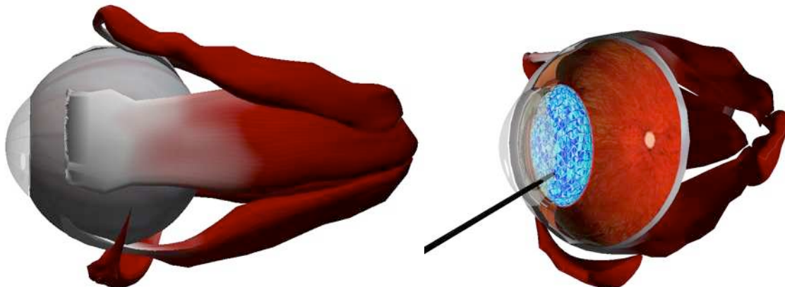
Figure 68: anatomical model of the eye in the cataract surgery simulation. (Left): the anatomical model in SOFA is rather detailed, and (Right) an illustration of a phacoemulsification device interacting with the tetrahedral mesh of the lens. The particular rendering of the lens is only for the purpose of showing the size of the tetrahedral elements.
