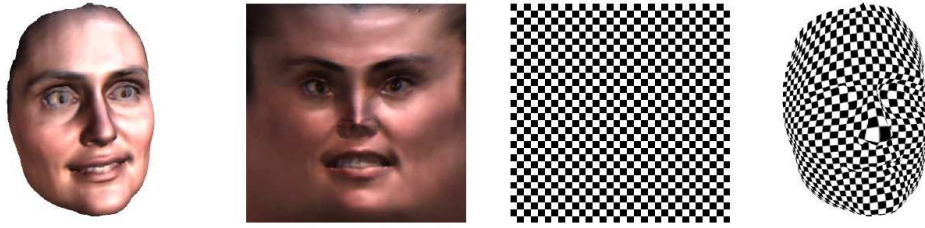
Figure 3.7 – Conformal mapping of a face surface S to its canonical domain D . From left to right: original textured surface, conformally mapped texture, canonical domain (u, v) coordinate system, conformal coordinate system S(u, v) (GY03).
