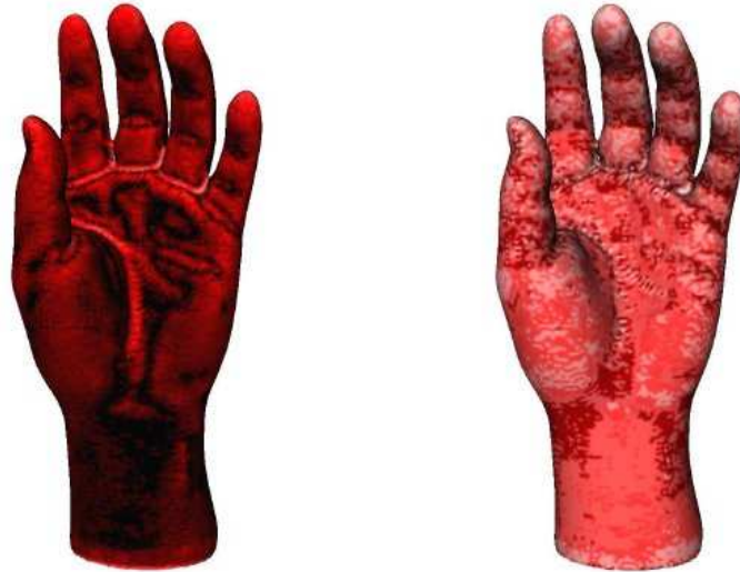
Figure 4.8 – The discrete mean curvature (left) and the discrete Gaussian curvature (right) computed on a triangulated surface.
