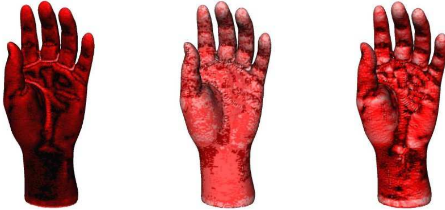
Figure 6.3 – Several curvature measurements on the hand triangulated surface: discrete mean curvature \kappa_{\mathcal{H}} (left), discrete Gaussian curvature \kappa_{\mathcal{G}} (middle) and curvature index \kappa_{\mathcal{I}} (KvD92) (right).
