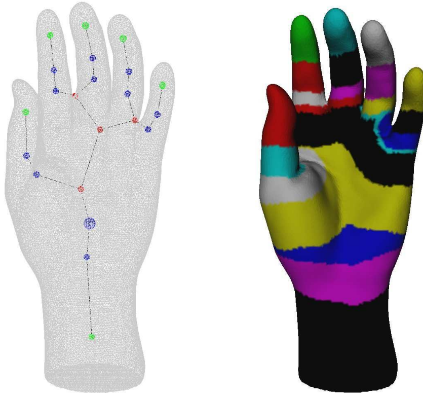
Figure 8.2 – Segmentation abstract graph and resulting segmentation.
