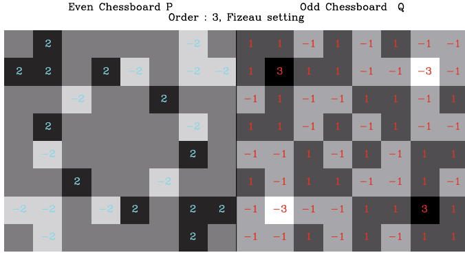
Fig. 4. The (P_n^*, Q_n^*) chessboards. The P_2, Q_2 chessboards from which they were built are in the top right corners. The 2k\pi or (2k+1)\pi phase shifts at \lambda_0 are indicated in the cells' centres by their 2k (blue) or 2k+1 (red) values. The value zero is not shown.
